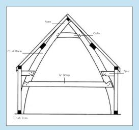
Figure B Cross section of a cruck-framed house. showing the curved 'cruck' blades.
