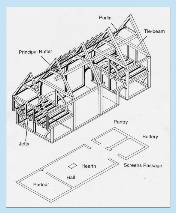
Figure A A typical medieval box-framed house, with an open hearth and a projecting first-floor jetty.
