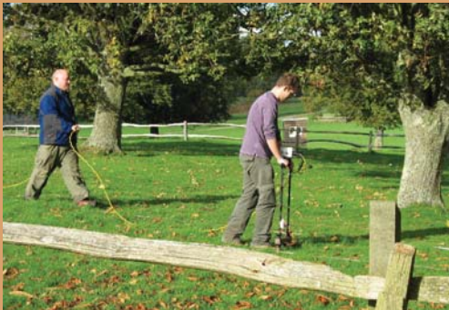
Figure A: Archaeologists from Archaeological Prospection Services of Southampton University carrying out a geophysical survey using a resistance meter in 2006. The probes of the resistance meter are clearly visible in this photograph, as are the measuring tapes which mark the survey grid.
