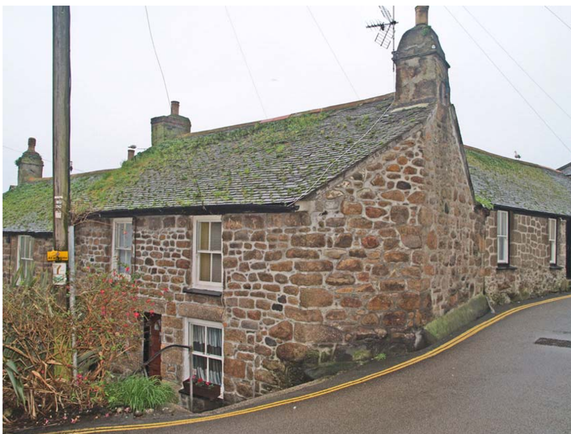
38. Context: houses west of Keigwins (17 th century dressed granite stack but rebuilt front wall)
